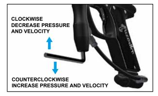
To increase the input pressure, use the allen wrench to turn the RockSteady Seat (P086) counterclockwise.
