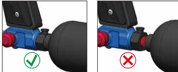
HPA / N2 Air tanks have enough force to become a projectile and cause serious injury or death if the regulator unscrews from the tank head.
